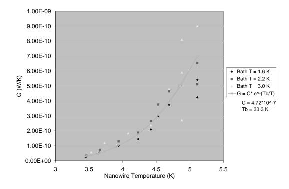
Figure 4. Thermal Conductance of the Nanowire. We estimate the effective thermal conductance G of the nanowire using a simple lumped element thermal model. The values of G we derive are consistent for all three bath temperatures. The conductance of the wire rises with wire temperature. This is to be expected since the unpaired electron density is a strongly increasing function of temperature near  $T_c$ .
