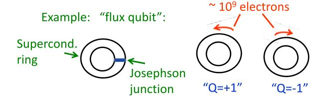
Existing experiments: if raw data interpreted in QM terms, state at  $t_{int}$  is quantum superposition (not mixture!) of states + and -.
