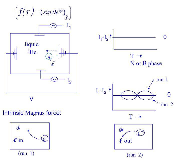
(Somewhat) unexpected effect: magnetic field can orient  $\ell$  – vector "in" or "out"! indicates coupling of  $\ell$  to field, i.e. <sup>3</sup>He is a weak orbital ferromagnet, with magnetic moment along ( $\pm$ )  $\ell$ .
