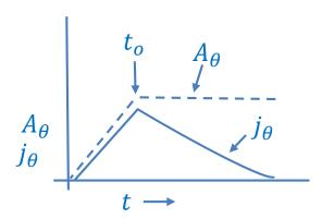
and in particular for  $t=t_o$   $v_\theta=-(e/m)A_f\Rightarrow j_\theta=-(e^2/m)A_f$  as in Quantum Mechanics case. However, this is not the lowest-energy state, so scattering by walls, etc. will reduce  $j_\theta$  to zero.
