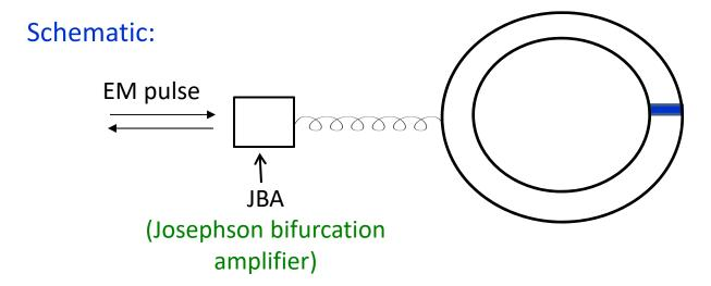
If we wish to measure Q at time t, inject EM pulse into JBA.
